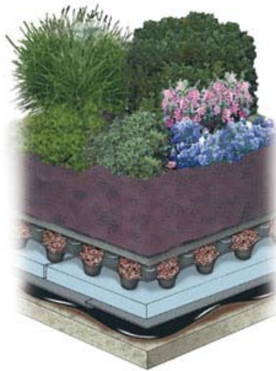
Intensive roofs use plants that require regular maintenance, such as watering and mowing. These roofs must be structurally stronger, and often serve as pedestrian recreational areas.
