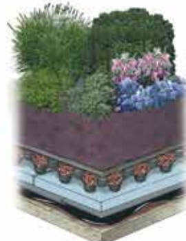
Intensive Garden Roof
