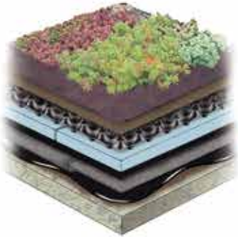
Extensive Garden Roof
