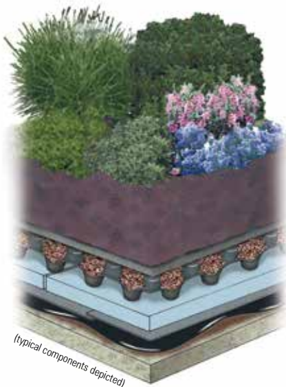
Intensive Garden Roof® Assembly
